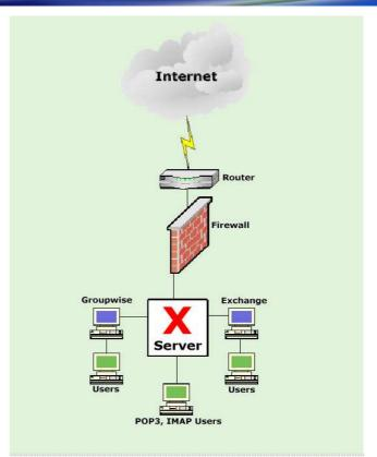
Typical network connection using MailXServer in a mixed environment.
